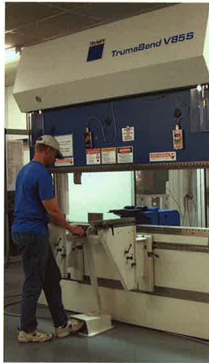
Figure 1: The back gauge "fingers" are moving into position.
