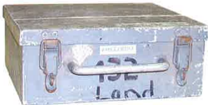
◀ This aluminum radio box was welded by Don Begneaud in 1978, and is still in use today.
