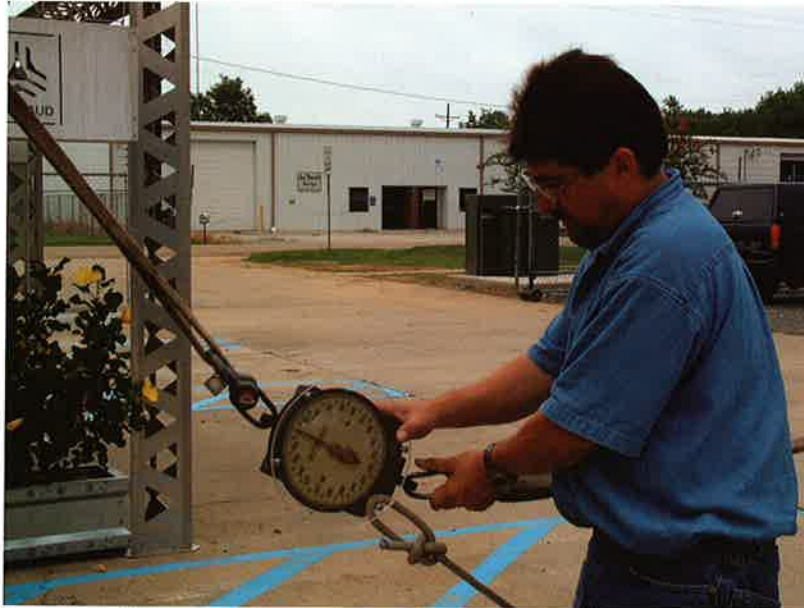
▲ Don attaches the slings to the scale used in the empirical testing. Don attached the slings to his forklift to complete the process of measuring the strength of the prototype. Various forms of empirical testing are used at BEGNEAUD to ensure the highest degree of quality and usability.
