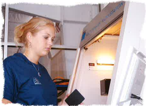
▲ Above: As part of her apprenticeship Natalie K ugler prepares a program for laser-etching at the TRUMPF Workstation 1200.
